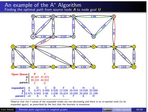
An example of the A\* Algorithm Finding the optimal path from source node A to node goal U
